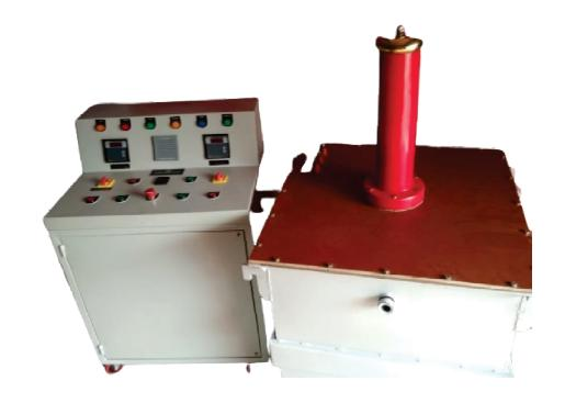
DC High voltage test set 0-200KV@
